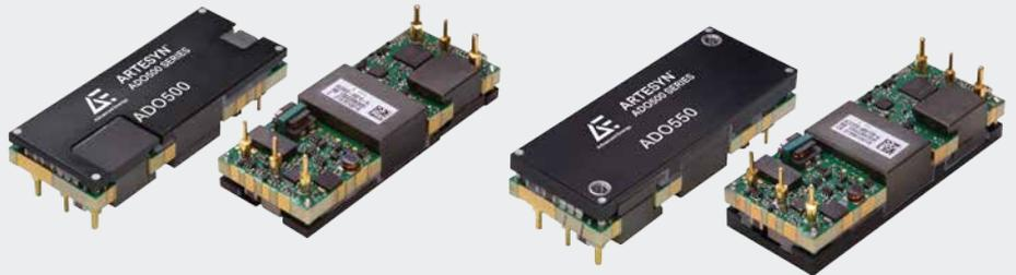
ADO500/550 series eighth-brick isolated DC-DC converters produce a single fully regulated 10 V output. Rated at 500/550 watts, these converters can deliver up to 55 amps output current and have no minimum load requirement. They have an input voltage range of 45 to 56 V and are primarily designed for use with standard 48 V supplies in computing and server applications, as well as regulated 48V supplies in communications equipment.
