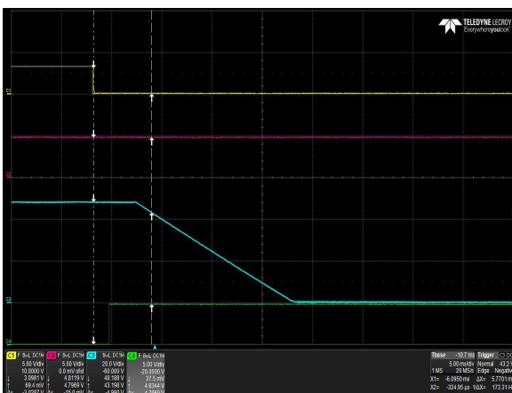
Figure 79: LCC600-48H-9P Turn Off Characteristic via INH_EN Load: I_O = 12.5A (48V), I_{SB} = 1.5A (5A) Ch 1: INH_EN Ch 2: V_{SB} Ch 3: V_O Ch 4: G_DCOK_C
