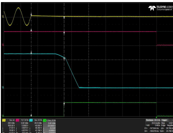
Figure 63: LCC600-48U-9P Hold-up Time Vin = 90Vac / 63Hz / 0° Load: I O = 12.5A (48V), I SB = 1.5A (5V) Ch 1: AC Mains Ch 2: V SB Ch 3: V O CH 4: G_DCOK_C
