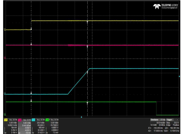
Figure 42: LCC600-36U-9P Turn-on delay via INH_EN Vin = 90Vac Load: I O = 16.7A (36V), I SB = 1.5A (5V) Ch 1: INH_EN Ch 2: V SB Ch 3: V O CH 4: G_DCOK_C
