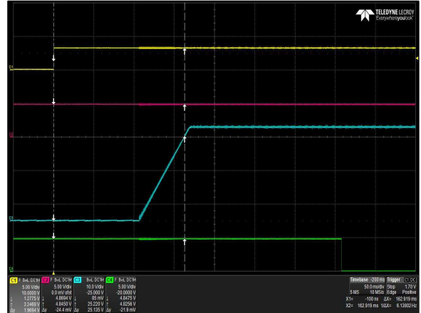
Figure 32: LCC600-28H-9P Turn-on delay via INH_EN Vin = 180Vac Load: I O = 21.5A (28V), I SB = 1.5A (5V) Ch 1: INH_EN Ch 2: V SB Ch 3: V O CH 4: G_DCOK_C
