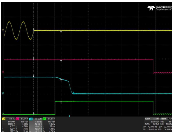
Figure 3: LCC600-12U-9P Hold-up Time Vin = 90Vac / 63Hz / 0° Load: Io = 50A (12V), I SB = 1.5A (5V) Ch 1: AC Mains Ch 2: V SB Ch 3: V O CH 4: G_DCOK_C
