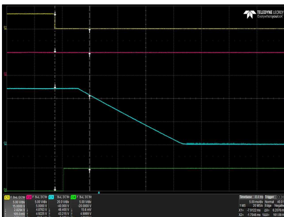
Figure 69: LCC600-48U-9P Turn Off Characteristic via INH_EN Load: I_O = 12.5A (48V), I_{SB} = 1.5A (5A) Ch 1: INH_EN Ch 2: V_{SB} Ch 3: V_O Ch 4: G_DCOK_C
