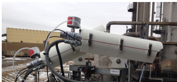
The ThermalSpection in its protective enclosure. Power, communication, and air connections are contained in a single hose.
